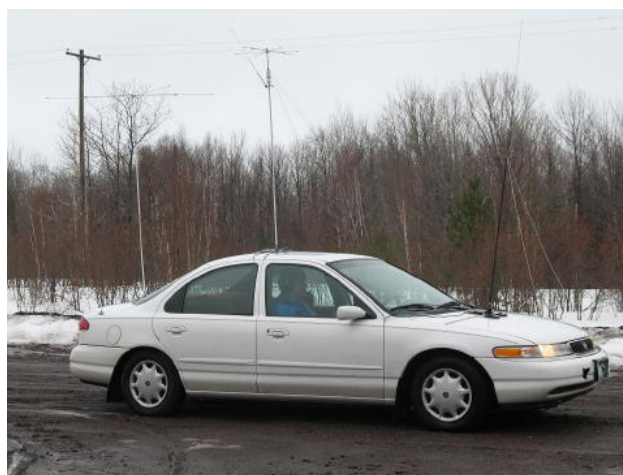
K8IR operating from snowy Keweenaw County. That's 80 meters on the trunk, 40/20 on the roof, and a 75 meter Hamstick on the hood. KG9GH Photo
